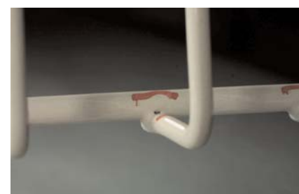
Diagram 4a: To avoid pore formation at the crossover area of two wires, the coating powder must be moved sideways in the sintering basin.
