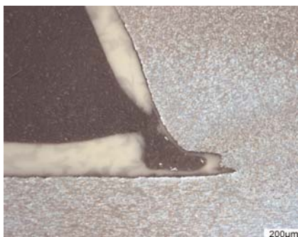
Diagram 4b: Pores may be starting points for underfilm corrosion and may ultimately necessitate high replacement costs.
